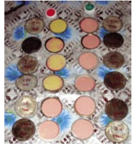
The result: Bacteria show yellow, pads without bacteria stay red in the Petri dish. Photo: CARE Yemen
